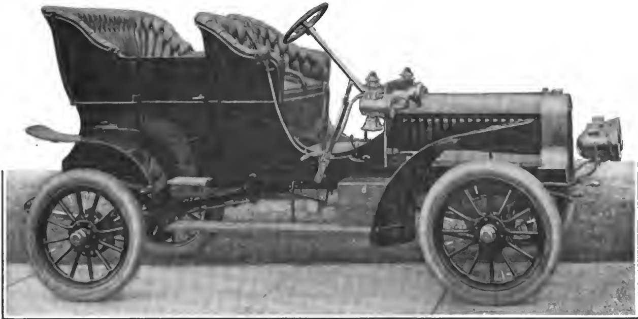
IROQUOIS MODEL D 25-30-HORSEPOWER, FOUR-CYLINDER TOURING CAR, WITH EXPANDING CLUTCH AND SLIDING GEARS.
